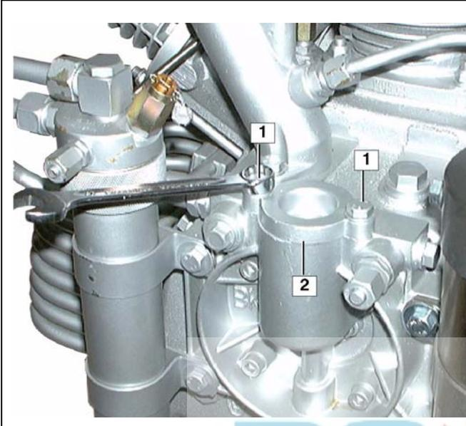
**Figure 3-6** Replacing the Oil Filter
